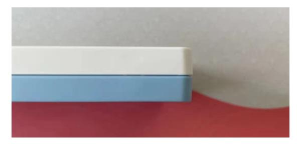
Please make sure that the internal parts are installed correctly and at the right places before screwing the top and bottom case together. The two cases shouldn't need any force to close together, so if you find yourself needing a lot of force to screw them together you should take another look at the internals.
