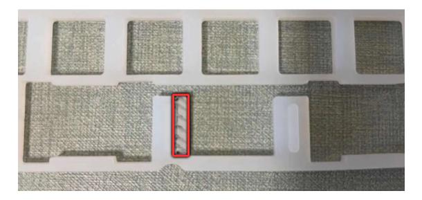
6. The optional **brass weight uses two different lengths of screws** to attach to the bottom case. The longer 8mm screws are used for part of the weight closer to the back, and the shorter 6mm screws are used for part of the weight closer to the front of the keyboard.
